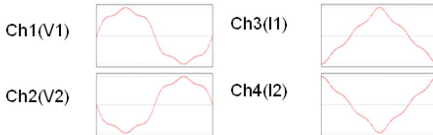
Figure 2: Sine Waveforms with 3rd and 5th Harmonics
