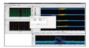
User-defined marker math allows time and frequency differences to be measured within or between channels.
