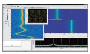
Spectrogram time windows positioned in time and frequency by marker placement.
