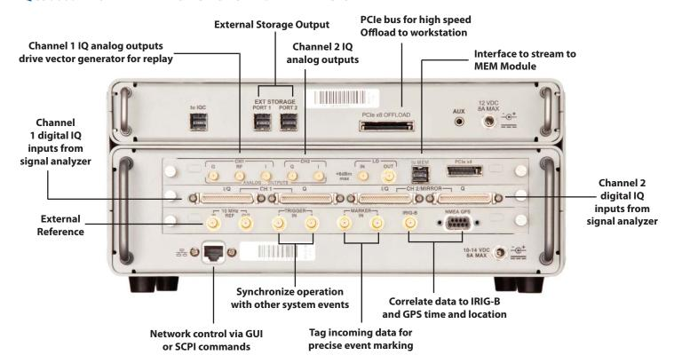
Rear panel interfaces include two analog I&Q Channel Outputs and two digital I&Q Channel Inputs, PCIe data offload, and IRIG-B and GPS inputs.
