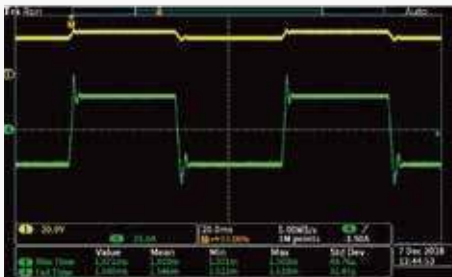
Control loop CV priority mode
