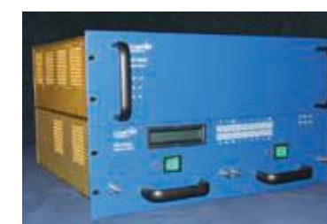
The standard remote control interface is RS-232 and RS-422. Ethernet control is available.
