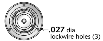
Coupling nut detail
