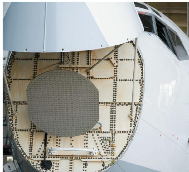
*Phased array and AESA radar systems are being retrofitted into both commercial and military aircraft. They employ dozens of low noise amplifier MMICs that are relied on for receiver sensitivity and optimal signal-to-noise ratio (SNR).*
