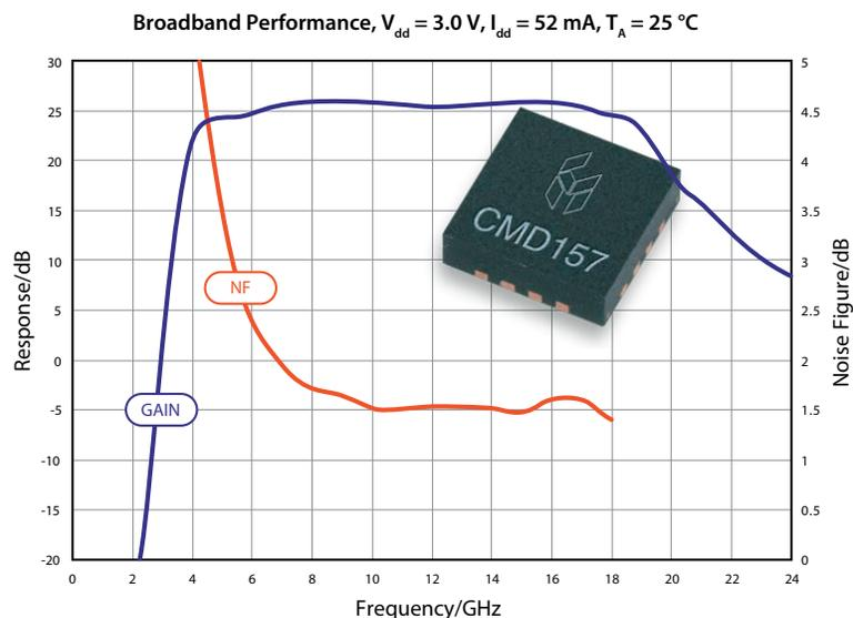
*This 6-18 GHz LNA exemplifies how gain flatness and gain stability over temperature are possible in a single device.*
