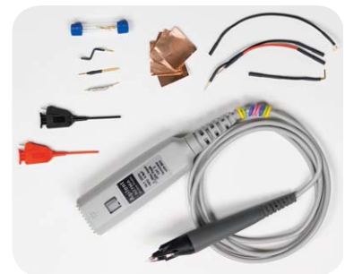
N2795A/N2796A 1/2-GHz active probe with AutoProbe interface, head light, and 1 M \Omega input Z
